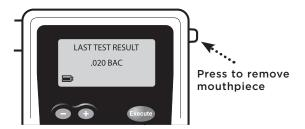
Press the **Function** button until the printer icon is displayed. The results of the last test will be displayed along with its test number at the lower left of the display.
