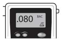
After the alcohol is graphed, the test result is displayed.
