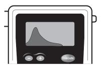
If the FC detects alcohol, the alcohol level is graphed and will be displayed before the result.
