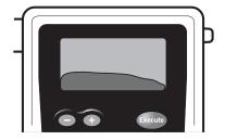
As the subject blows into the mouthpiece, the FC20 will show a graph of the breath flow on the display, as well as showing the amount of liters. Liters are shown in the upper left corner.
