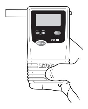
Press and hold the **Power** button on the bottom of the front of the unit until it beeps. The FC20 performs an automatic internal diagnostics check when turned on.
